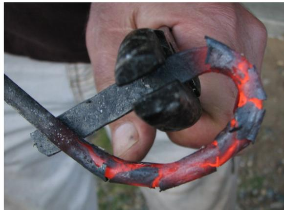
(5) Cut off the extra stock, and straighten and/or smooth out any waviness in the 'D.'
