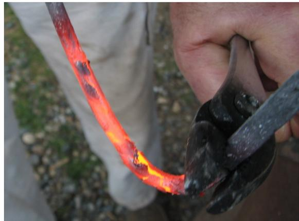
(4) Heat and bend the next section of the steel stock into a gentle curve to make a 'D' shape. The straight part of the 'D' is the striking edge, and the curved part is the handle.
