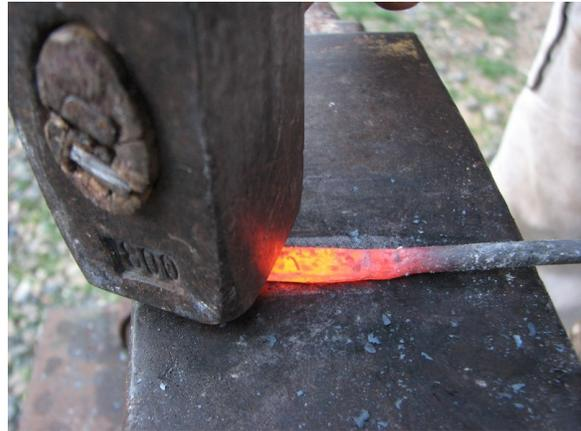
(2) A straight, flattened and narrowed striking edge is the easier to get good hot sparks from. So, heat one end of the steel stock, then place it on the anvil, and use the hammer to flatten the last 1½ to 2 in / 4 to 5 cm from the end. Make it a little over 1/16 in / 2 mm in thickness. Re-heat as necessary. Finish by making this section as straight and even as possible. One of the thin sides of this section will be the striking edge.
